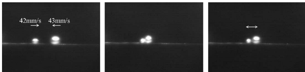
Fig. 3. Bubble collision and detachment.
