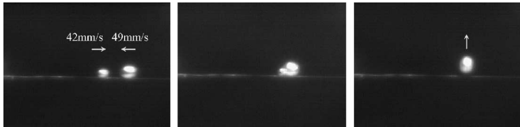
Fig. 4. Bubble collision, coalescence and departure.
